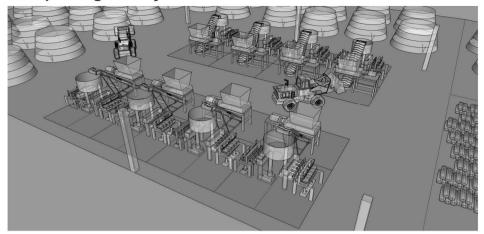
Briquetting and/or Chipping Facility for briquetting and/or chipping sorted woods Modular expandable, 1 ton/h modules
